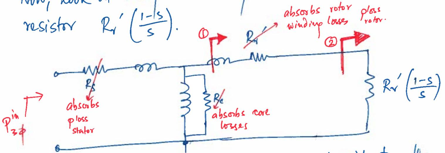
Q. What's the power absorbed by the circuit to the right of the arrows at ① and ②?
