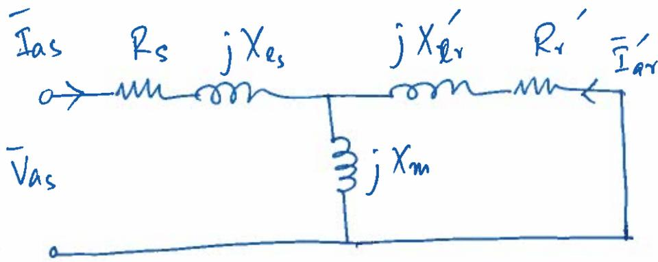
$R_s$  = Resistance of stator
