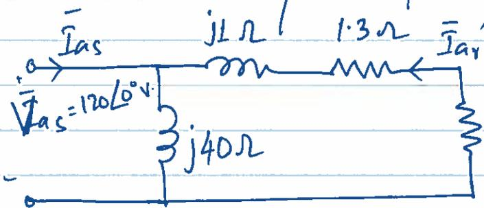
$$R_r' \left( \frac{1-s}{s} \right) = 1.3 \times \left( \frac{1-0.045}{0.045} \right) \Omega = 27.6 \Omega$$
